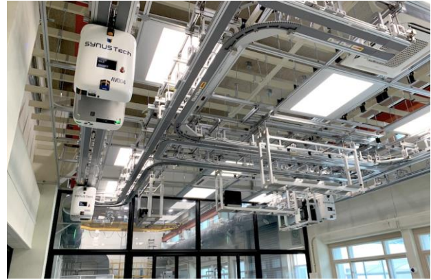
Figure 1. OHT vehicle used in semiconductor factories.
